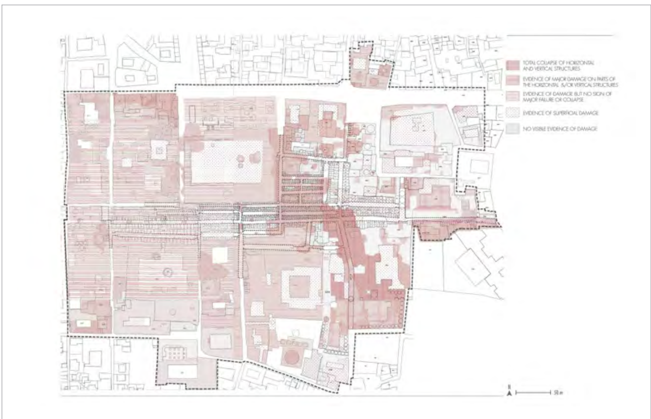
Fig. 4. The Central Commercial Zone: the levels of damage based on the assessment carried out by AKTC in 2017, (courtesy of AKTC)
